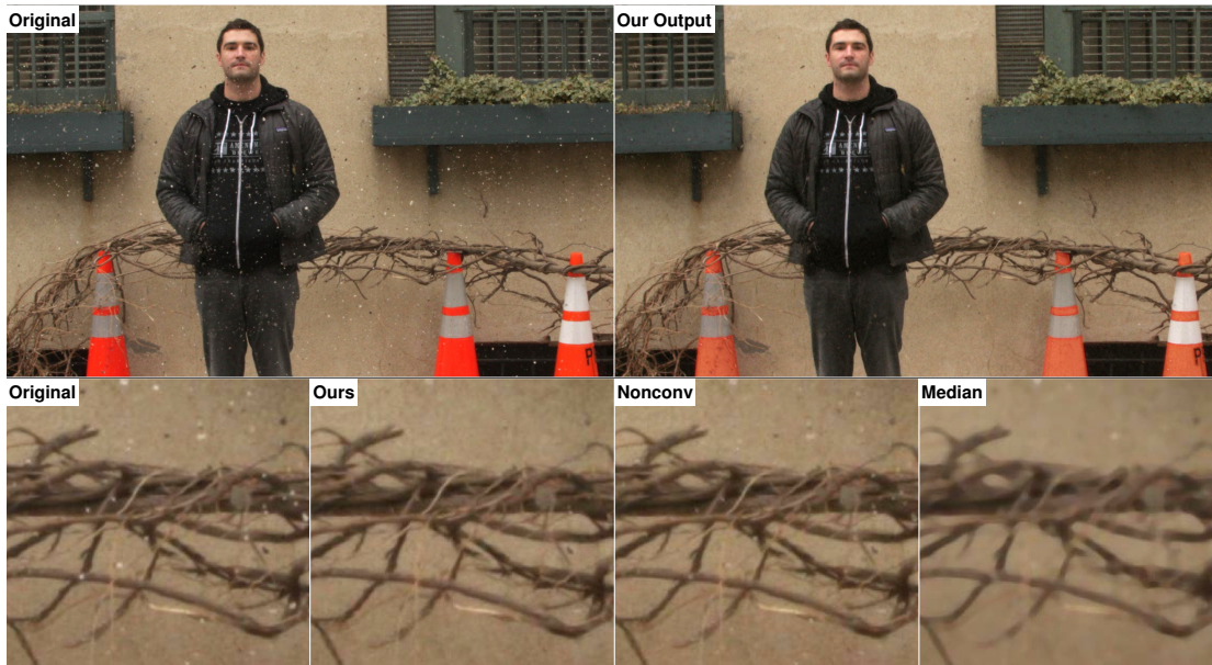
Figure 4.5: Example image containing dirt, and the restoration produced by our network. Note the detail preserved in high-frequency areas like the branches. The nonconvolutional network leaves behind much of the noise, while the median filter causes substantial blurring.
